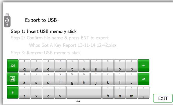
4. Insert a USB memory stick into the slot on the system.
