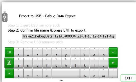
iii) After inserting a USB stick, you can rename the file. Once finished click the enter button.
