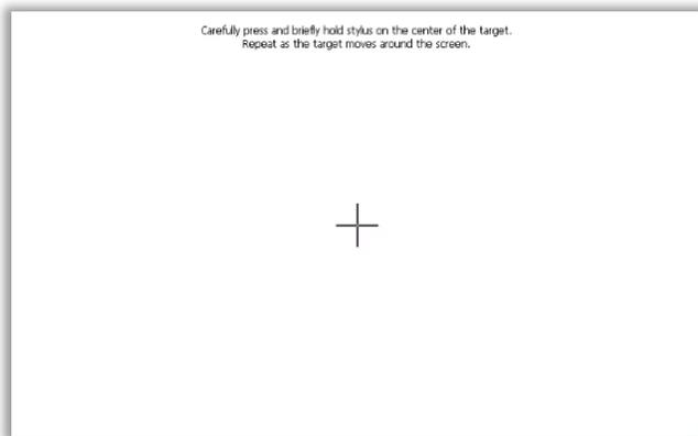
Once the calibration procedure is finished, the following screen is presented. Tap the screen once more to register and save the calibration data. If you do not tap within 30 seconds then the new calibration data will not be saved.
