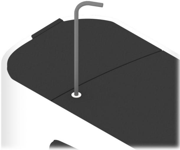
2. Remove the cover plate and screws.
