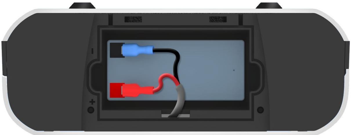
5. Replace the cover and screws using the 2mm Allen Key.
