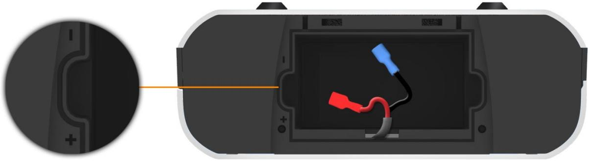
4. Connect the battery to the battery cable. Use the connection code in the section above for guidance.
